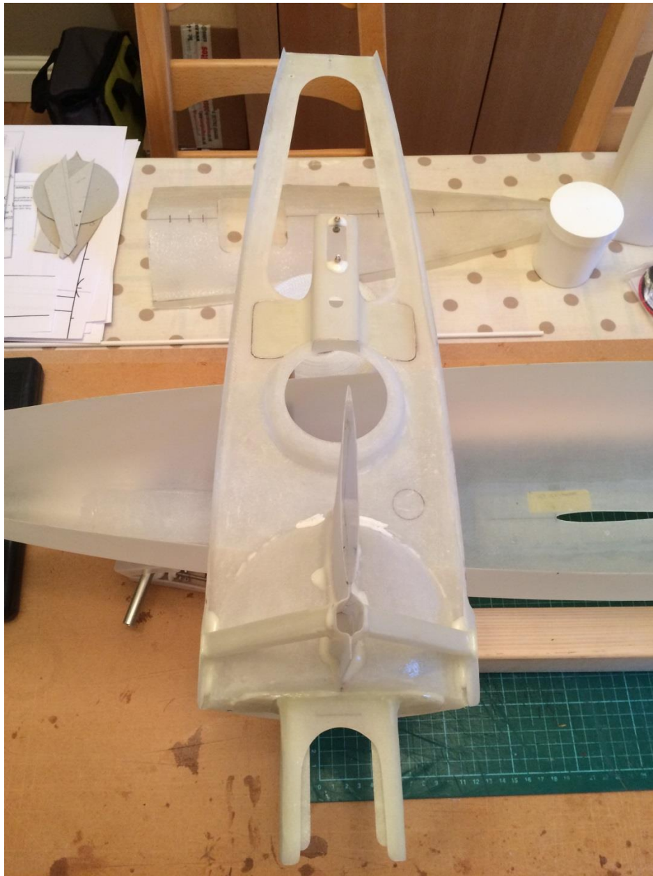
Underside of Rear Deck showing Fin Box, support beams, Winch Tray and Rudder Servo Mount
