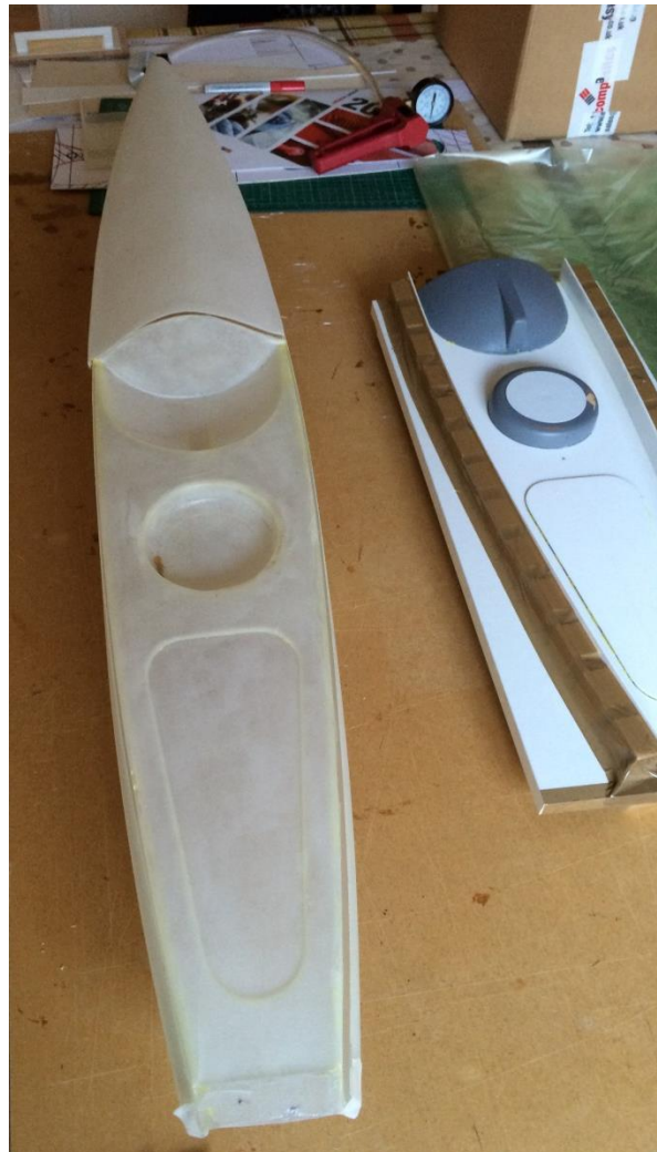
Hull, Rear Deck and Foredeck before trimming
