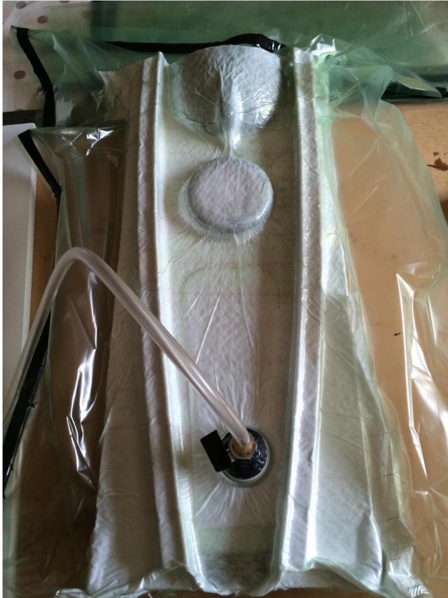
Vacuum bagging of the Rear Deck
