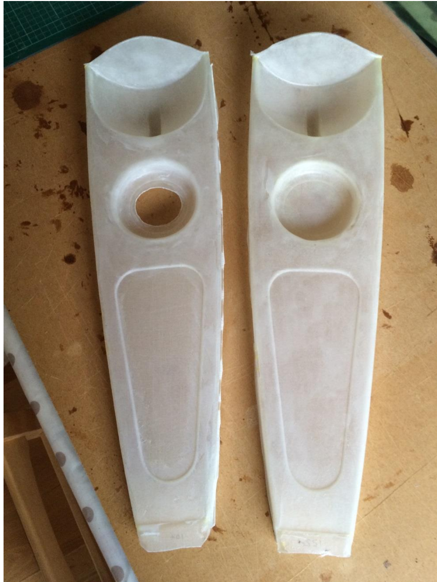
Rear Deck mouldings fresh from the plug!
